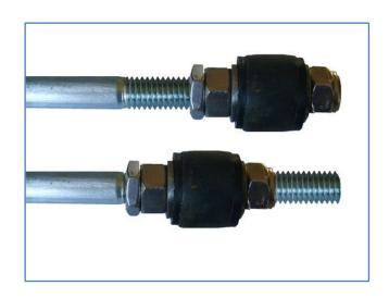
Reconnect the 22mm tube by sliding it over the assembly and reconnected to the brass T-piece; do the nut up firmly. In this mode a 13mm box spanner will be required to adjust the pressure on the silicone plunger.
